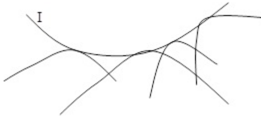
Fig. 7.1 The envelope of a family of curves
